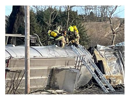
6.4: <u>EPU:</u> Specialist clay putty utilised to stem leak of substance from ruptured tanker. Boom systems and chemical absorption mats/socks used to contain substance from entering drains and open water source.
